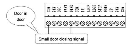
4. Infrared sensor connection. Please make sure the connected infrared sensor is "NO". System default type is "NO". To change it into "NC", please set it under <u>parameter setting menu 16.</u> Infrared sensor type selection. Connect to "24V", "COM", and "IR" ports accordingly.
