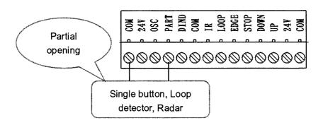
3. Small door interlocking (door in door). If there is a smaller door inside the main door, connect closing signal line of the smaller door to "DIND" and "COM" ports. Under which if the smaller door is opened, the main door will not work; The smaller door is closed, then the main door can work.
