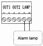
9. Relay output. Please refer to parameter setting menu 13. Relay output, two relays' output ports are available under the system, each has 6 kinds of output types for choosing.
