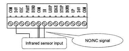
5. Loop detector or radar connection. Please make sure the type of connected loop detector or radar is "NO". System default type is "NO". To change it into "NC", please set it under <u>parameter setting</u> <u>menu 17.</u> Loop detector type selection. Connect to "24V"、 "COM" and "LOOP" ports accordingly.
