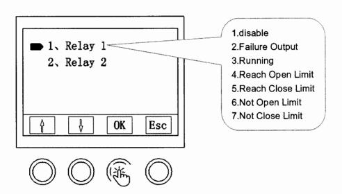
For example: Dual machine interlocking. Select 7. Not Close limit position output for relay 1 of both control units
